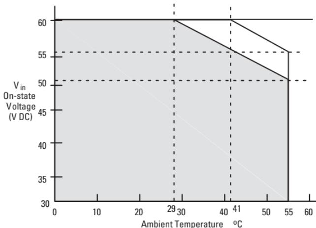
The area within the curve represents the safe operating range for the module under various conditions of user supplied 48V DC supply voltages and ambient temperatures.
