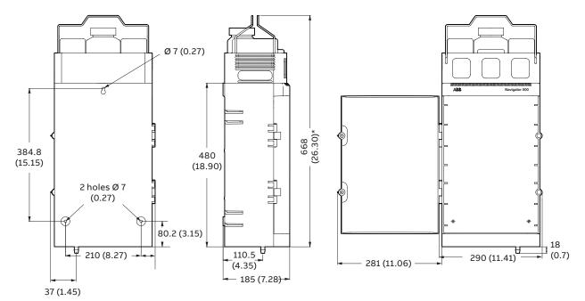
\*When installing, allow a further 60 mm (2.36 in.) min. to remove the bottle carrier assembly, or 135 mm (5.31 in.) min. to remove the calibration solution bottle from the carrier.
