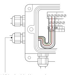
Additional serial cable connections to multiple wet-sections
