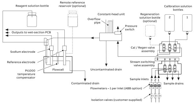
Figure 2 Schematic flow diagram – sodium multi-stream
