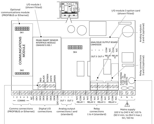
Wet-section terminal connections
