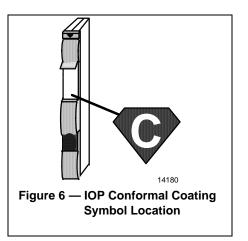
**Note:** Boards installed and maintained in a G1 (mild) control room environment (defined by the ISA Environmental Severity Classification) do not need this added protection.
