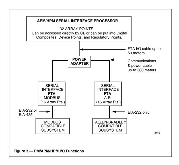
The Modbus SI FTA supports Modbus RTU protocol and uses either EIA-232 or EIA-422/485 communications, including multidrop configurations. The Allen-Bradley FTA supports DF-1 protocol and uses only EIA-232 communication.
