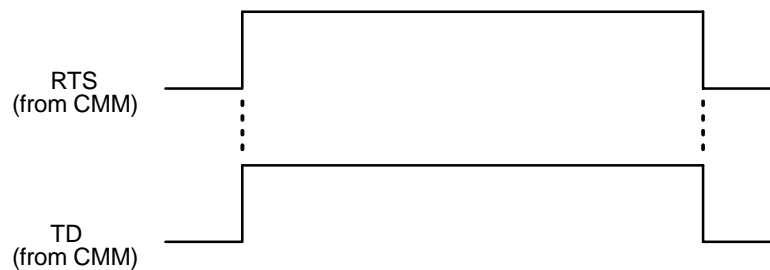
Figure 2-7. Flow Control = NONE, MODEM TURNAROUND DELAY=0
