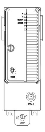
The CI865 expansion unit contains the CEX-Bus logic, ControlNet bus logic, CPU and a DC/DC converter that supplies appropriate voltages from the +24 V supply, via the CEX-Bus.
