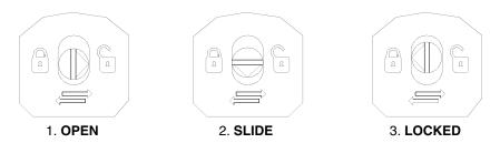
Figure 17. Baseplate Locking Device
