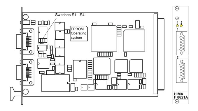
The coprocessor module has its own microprocessor HD 64180 and operates with a clock frequency of 10 MHz. It contains mainly the following functions:
