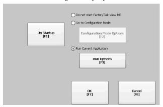
2. Press the On Startup button to select Run Current Application.
