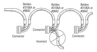
Attach the connector to a Belden 3106A or 9842 cable as shown <u>Figure 17</u> or <u>Figure 18</u>.
