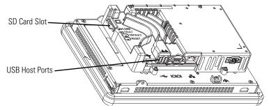
To remove the SD card, press on the card to release it, then pull it out. To remove a USB flash drive, gently pull it from the port.
