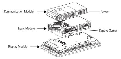
**5.** Carefully lift the logic module away from the terminal and turn over to expose the circuit board.
