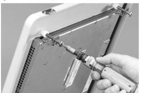
6. Tighten the mounting clips screws to a torque of 0.90...1.1 N•m (8...10 lb•in) by using the specified sequence, making sure not to overtighten.
