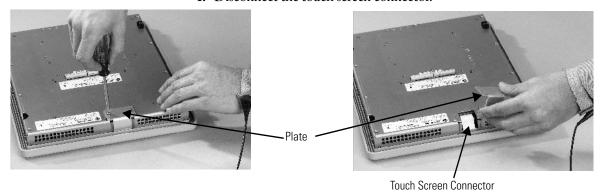
**5.** Remove the screws from the back of the display module.
