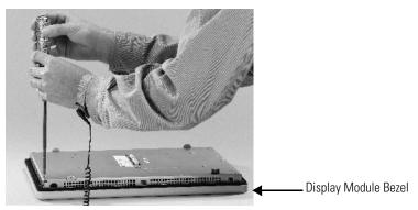
6. Remove the sealing gasket.
