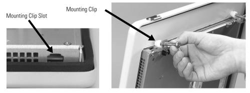
4. Slide the ends of the mounting clips into the slots on the terminal.
