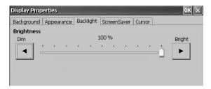
**TIP** When the backlight is in Overdrive mode, the backlight brightness level cannot be adjusted.
