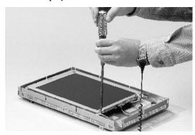
**4.** Lift the LCD display and detach the display connector from the circuit board.
