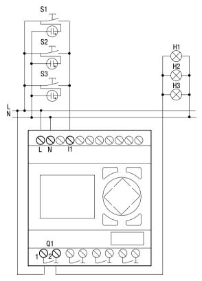
Figure 79: Stairwell lighting with the logic relay
