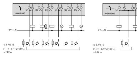
Figure 28: Relay outputs CL-LMR and CL-LER.20
