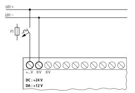
Figure 9: Supply voltage to DC basic unit
