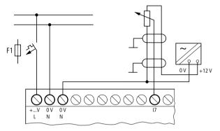
Figure 20: Analog setpoint potentiometer with own power feed
