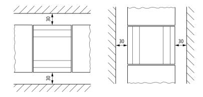
Figure 4: Clearances from the logic relay
