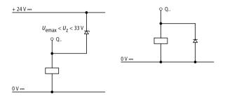
Figure 33: Inductive load with suppressor circuit
