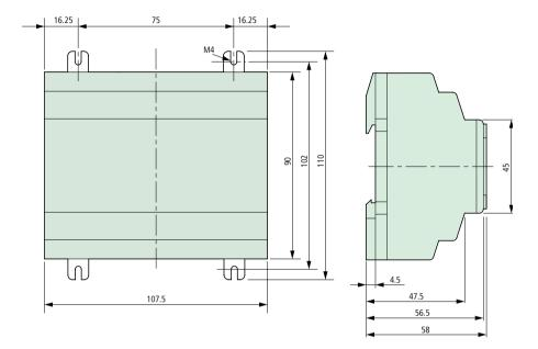
Figure 95: Dimensions CL-LMR/CL-LMT in mm (specifications in inches see table 34)
