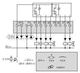
Figure 31: Transistor outputs CL-LMT
