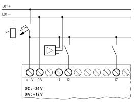
Figure 17: Connect digital inputs CL-DC1 and CL-DC2
