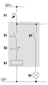
Figure 36: Lamp controller with relays
