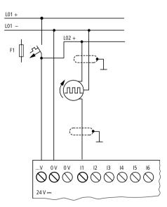
Figure 25: Connecting high-speed counters and frequency generators
