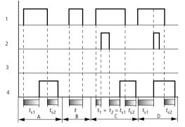
Figure 66: Signal diagram timing relay, on and off-delayed 1
