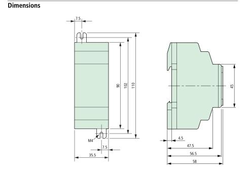
Figure 93: Dimensions CL-LEC.Cl000 and CL-LER.20 in mm (specifications in inches see table 34, page 253)
