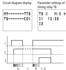
Figure 72: Function of the circuit
