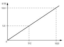
Figure 47: Resolution of the analog inputs
