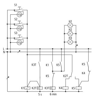
Figure 78: Conventional stairwell lighting
