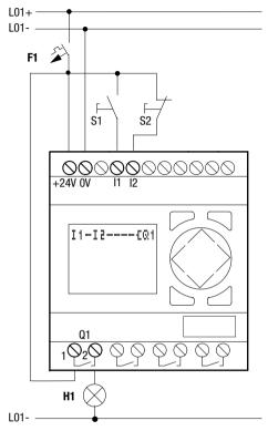
Figure 37: Lamp controller with logic relay
