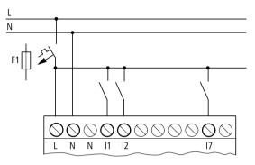
Connect digital AC inputs to the basic unit
