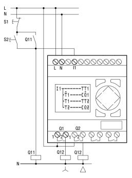
Figure 74: Star-delta circuit with the logic relay
