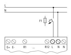
Figure 8: Supply voltage to AC basic unit
