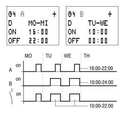
Figure 61: Time overlaps signal diagram
