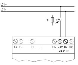
Figure 10: Supply voltage to DC expansion unit
