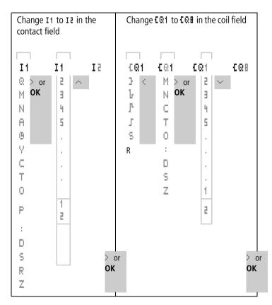
The logic relay will leave Entry mode when you press < > or **OK** to leave a contact field or coil field.
