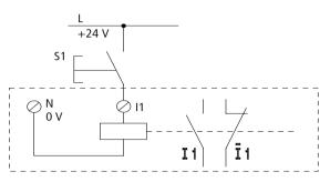
Figure 11: Connecting the inputs
