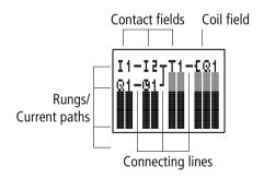
• Connections are used to produce the electrical contact between switching contacts and the coils. They can be created across several rungs. Each point of intersection is a connection.
