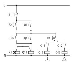
Figure 73: Star-delta circuit with conventional contactors
