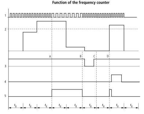
Figure 55: Signal diagram of frequency counter
