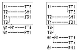
Figure 80: CL circuit diagram for stairwell lighting
