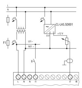
Figure 19: CL-AC1 analog input, connection of reference potentials
