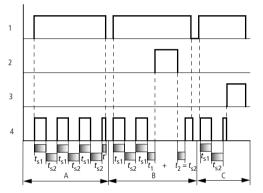
Figure 71: Timing relay signal diagram, flashing
