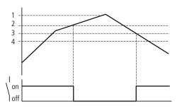
Figure 48: Signal diagram of analog value comparator in Less than mode
