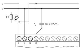
Figure 15: Increasing the input current
