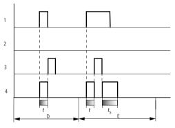
Figure 70: Signal diagram timing relay, pulse shaping 2
