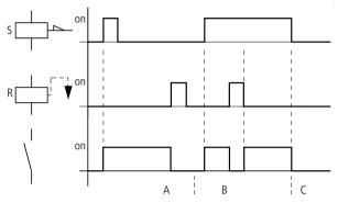
Figure 44: Latching relay signal diagram
