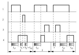
Figure 67: Signal diagram timing relay, on and off-delayed 2
