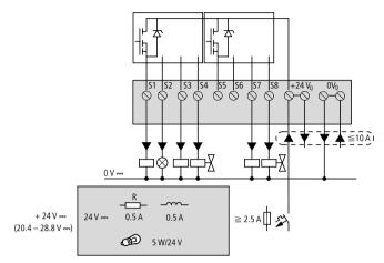
Figure 32: Transistor outputs CL-LET.20DC2
