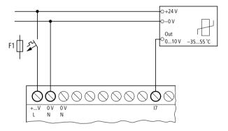
Figure 23: Connection of the temperature sensor, analog input
