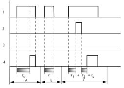
Figure 62: Signal diagram of timing relay, on-delayed (with and without random switching)
