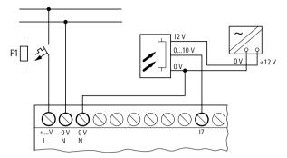
Figure 22: Connection of a brightness sensor, analog input
