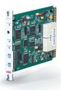
The speed input module 70EI06a processes the pulse signals from a speed sensor, calculates the speed of the turbine, then based on user defined criteria outputs the speed measurement and other indications to the P13 local bus. The module also provides two relay contacts for protection applications, e.g. electrical 2003 voting.
