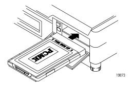
If the computer is configured properly, your sound/speaker is enabled, and you installed the PCMK card successfully, you hear multiple tones when you insert a card or boot the computer. If you have two PCMCIA cards, there are 2 sets of tones, one for each card.
