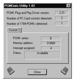
If you are using a 16-bit communication package such as WinLinx or INTERCHANGE software, the socket number you use when configuring the software is one less than the number specified by PCMKINFO. This is because Microsoft changed the numbering convention when going from Windows 3.x to Windows 95 operating systems.
