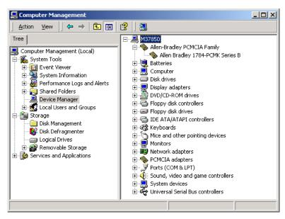
We recommend using only one card at a time. If you insert two PCMK cards, only one card will be available for use. The Device Manager window looks like this:
