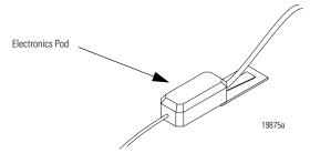
2. Position the assembly on the computer so the narrow end of the wedge is closest to the PCMCIA slot. When you find the best location for the wedge, use a pencil to mark the location on the computer.
