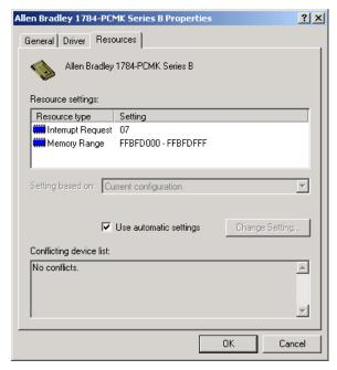
The majority of the time, we recommend that you use the automatic settings. The operating system assigns an interrupt and memory location for you. An interrupt must be assigned to the 1784-PCMK card. Verify that there is an interrupt assigned and no resource conflicts display in the Conflicting Device list.
