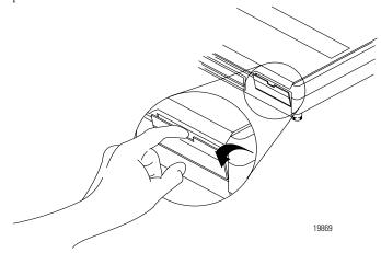
2. Grasp the PCMK card by the edges with the PCMK logo facing upward and the 68-pin connector facing into the PCMCIA slot.
